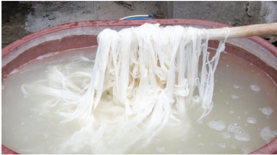
SE HUMEDECE LA CORTEZA THE TREE BARK IS MOISTENED
